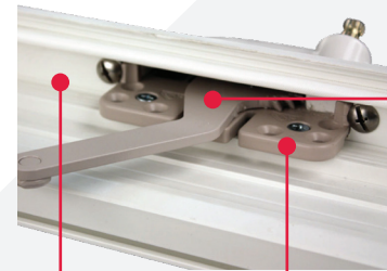
The operator is anchored to the window on 2 planes - the base and the tower, preventing handle tilting typically seen in other windows.
